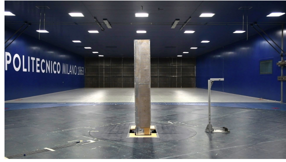
(b) Model with porous mesh installed.
